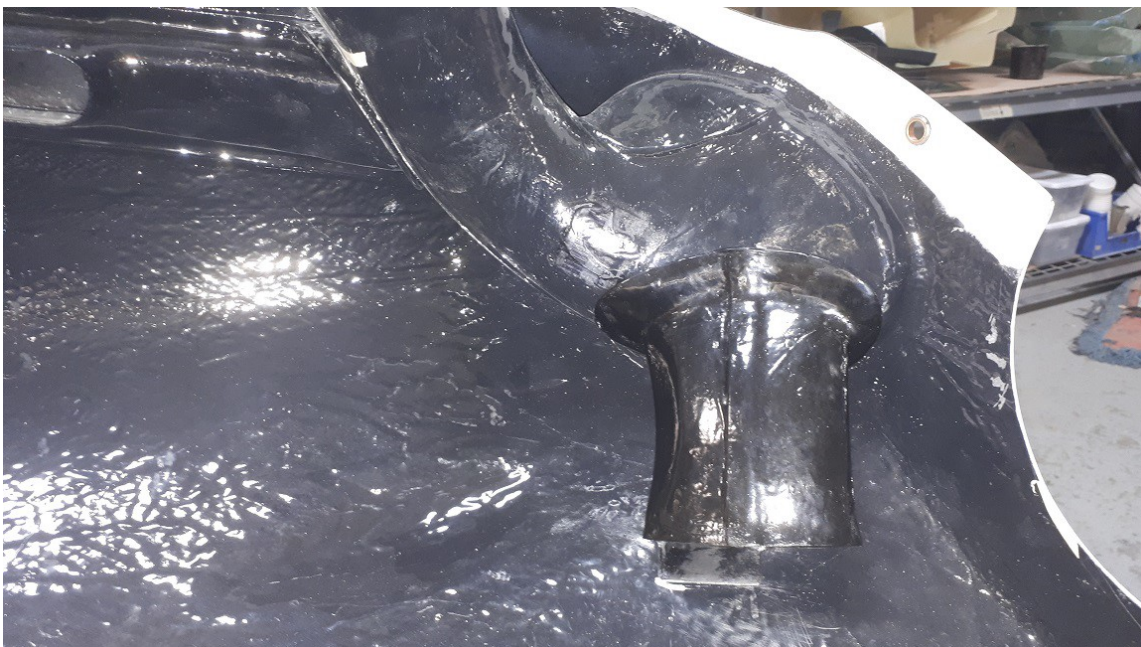
Figure 4. Position of the new secondary air duct (closer view).
