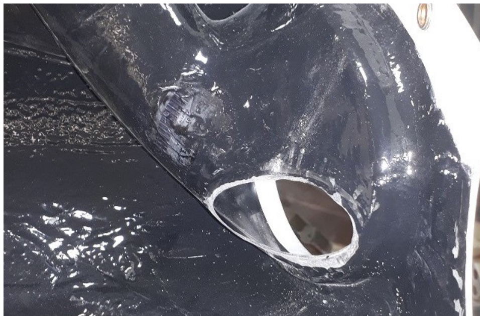
Figure 2. View after removing the secondary air duct, looking towards the top surface of the cowling.
