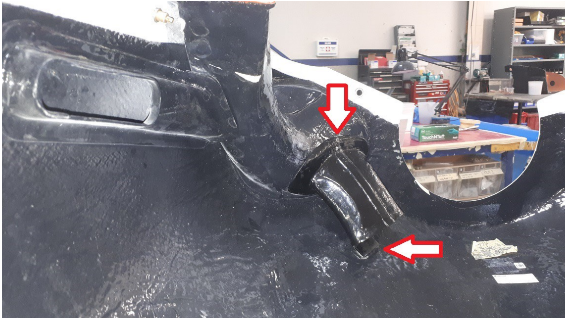
Figure 3. Position of the new secondary air duct. Areas to be bonded shown by arrows.
